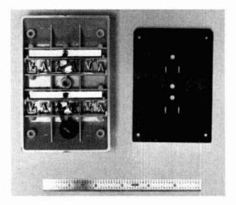
fig. 3. Interior view of the accessory outlet box with one MOV installed across the AC hot and neutral lines. Note the protective sleeving on one of the MOV's leads.
